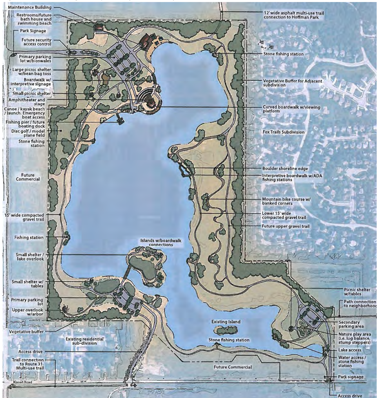
Figure 9. Schematic design concept for Cary Lake at Rotary Park
