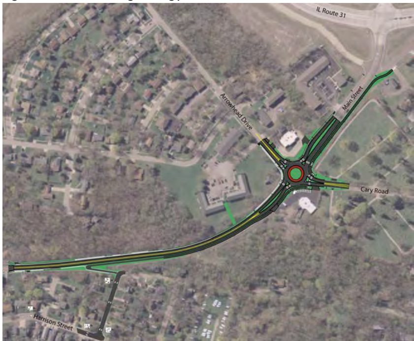
Figure 12. Roundabout engineering plan
