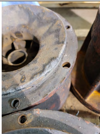
Mating bowl faces are deteriorated due to graphitization
