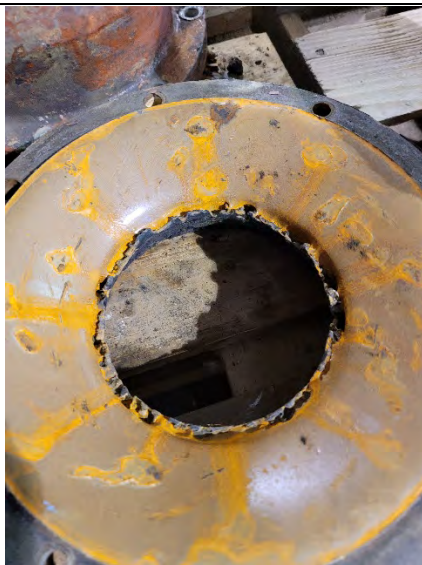
Erosion of Bowl face, heavy pitted
