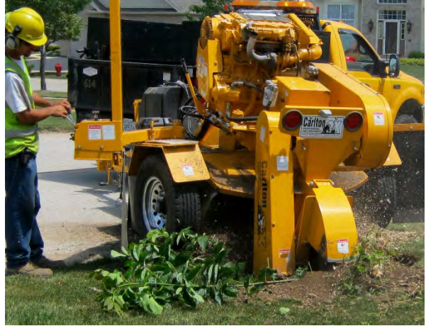
Public Works staff grinds a stump from a parkway tree in a residential area
