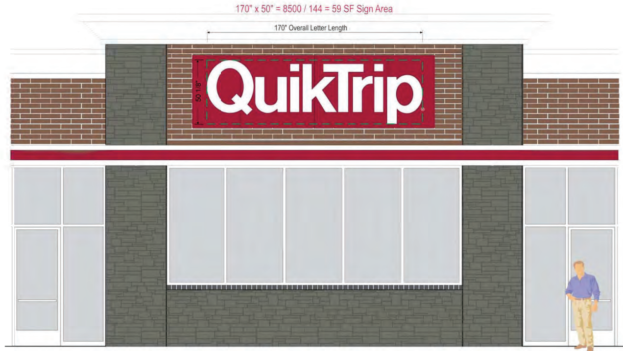
Front View - Sign Type CL-60F-LD - Flat Front Aluminum Wall Sign Projected Channel Letters with White LED Illuminated LD Poly Faces & Red LED Halo
